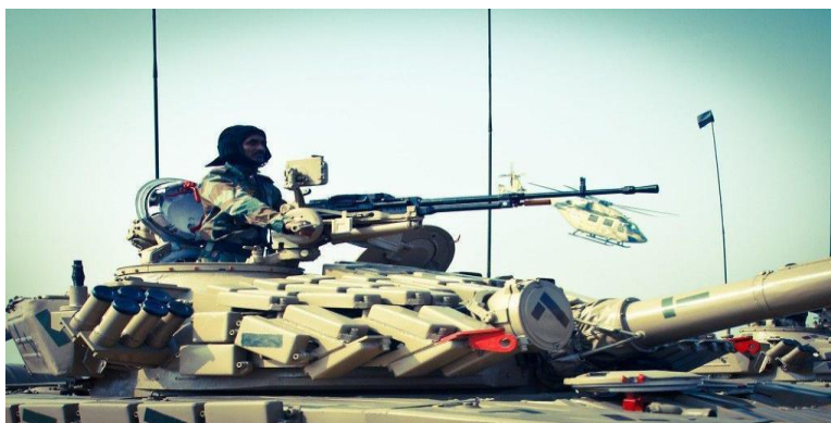
Figure 2: NSVT mounted on Tank
